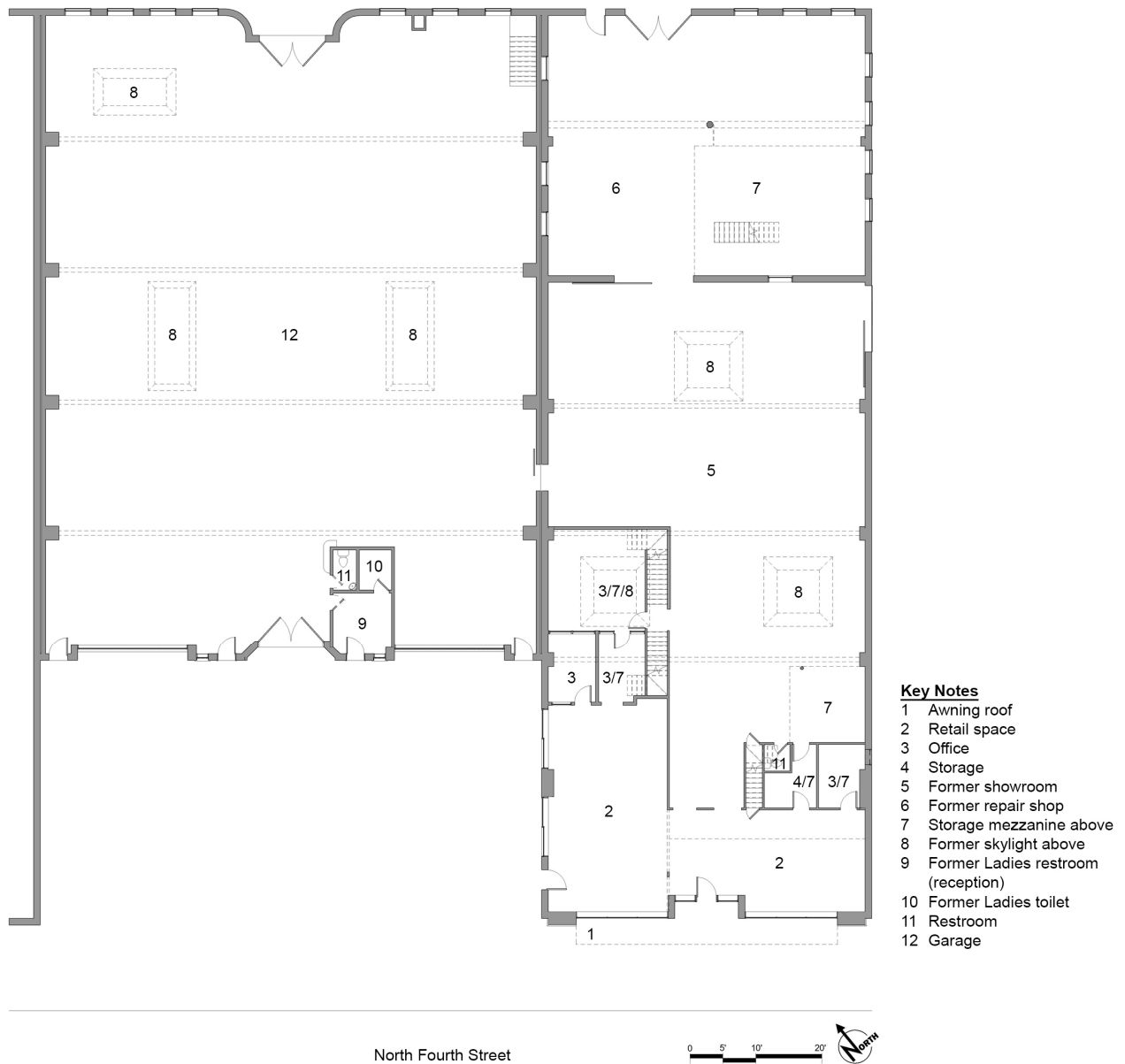
Figure 1: Floor Plan of Lyons Garage (left) and Lyons Auto Company (right) with key notes, 2020. Source: Measured and drawn by author.
